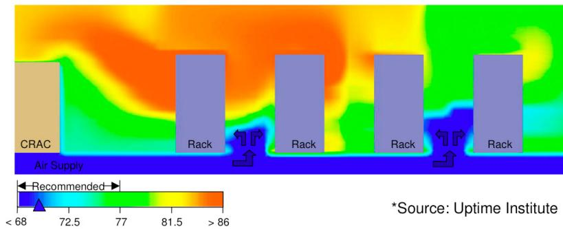
**Figure 3:** Air Flow in a Traditional Data Center
