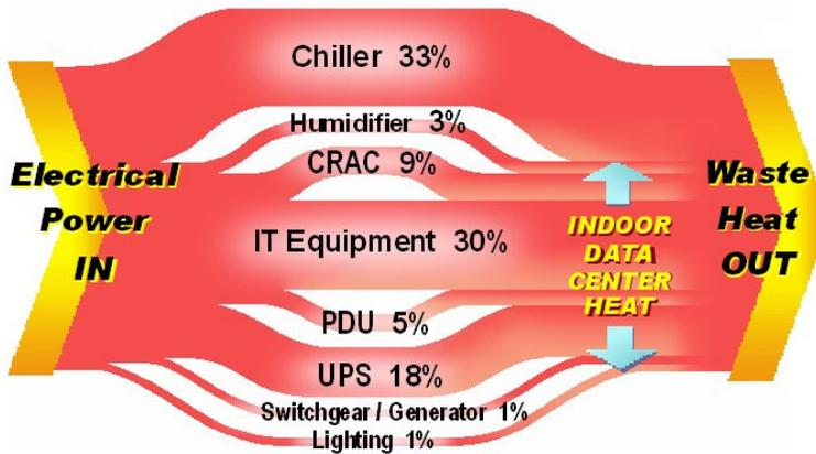
Figure 2: Electrical Efficiency in a Data Center (Source: APC)
